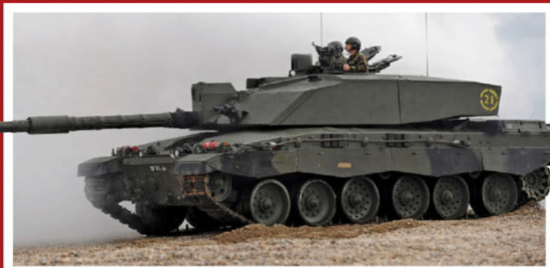
Below: A Challenger 2 aims its L30A1 120mm main gun at a distant target
